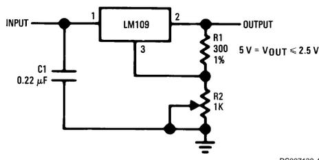
\*Required if regulator is located more than 4" from power supply filter capacitor.
