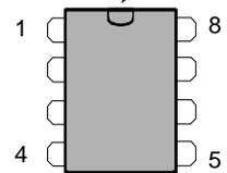
Pin numbers are placed on the connections to the I.C. in circuit diagrams.
