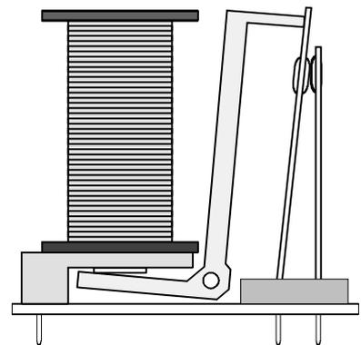
When energised, the coil becomes an electro magnet, attracting the metal lever, pushing the contacts together.
