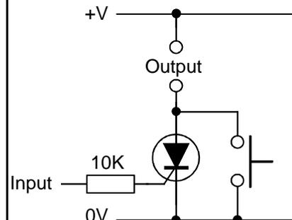
Once an input is sent to the gate, the thyristor conducts and latches on. The only way to switch off the output is either disconnect the power or short out the thyristor using a push switch. Some thyristors can switch up to 30 Amps.
