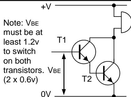
Note:  $V_{BE}$  must be at least 1.2v to switch on both transistors. ( $2 \times 0.6v$ )
