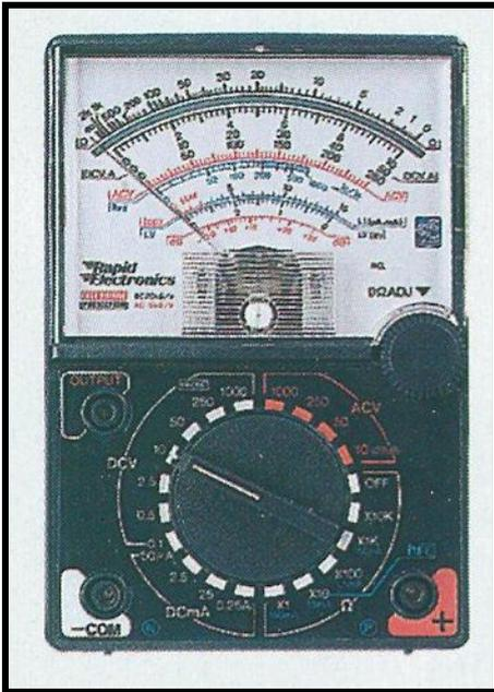
There are two main types of Multimeter, Analogue (shown left) and Digital (shown right). Digital meters are very accurate but analogue meters can show a slowly changing reading more clearly.
