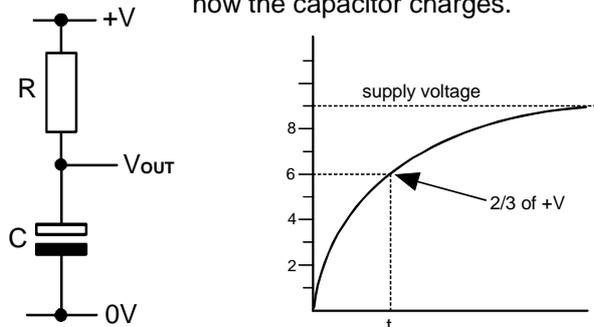
The formula  $t=CR$  is used to calculate the time it takes for the capacitor to charge to 2/3 of +V.
