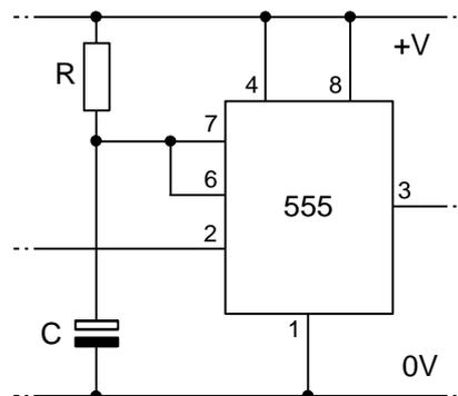
The 555 timer can be connected as a monostable. The timing is set by R and C. The formula is  $t = 1.1CR$
