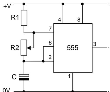
The output is known as a **square wave** with equal **mark/space** ratio.
