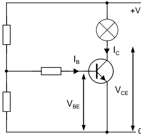
The diagram shows the basic current flow and voltages when a transistor is in use. These are called parameters.
